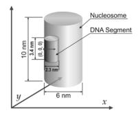
Figure 1. Geometrical set-up of the Monte Carlo simulations. The DNA segment and the nucleosome were embedded in a water cube of 150 nm edge length. The particle beam was incident on the surfaces on both cylindrical targets and directed along the x-axis.
