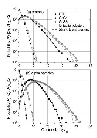
Figure 11. Probability distribution of ionisation cluster size and DNA strand breaks in the DNA segment for 300 keV protons (a) and 1 MeV alpha particles (b), calculated by means of the PTB and Geant4-DNA MC codes.
