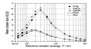
Figure 3. Mean ionisation cluster size  $M_1(Q)$  as a function of incident electron energy *T* obtained in the DNA segment (DNA) and the nucleosome (Nuc) by the PTB simulation and Geant4, using the Screened Rutherford (G4SR) and the Champion model (G4Ch) for elastic scattering.
