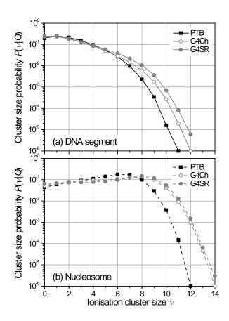
Figure 2. Probability distribution of ionisation cluster size P(v/Q) in the DNA segment (a) and the nucleosome (b) obtained for incident electrons of 200 eV, calculated by means of the PTB and Geant4 MC codes by using the Screened Rutherford (G4SR) and the Champion model (G4Ch) for elastic scattering. Statistical error bars are not shown; for probabilities of approximately 10<sup>-5</sup> and higher, the uncertainties are within the symbols. Below this value
