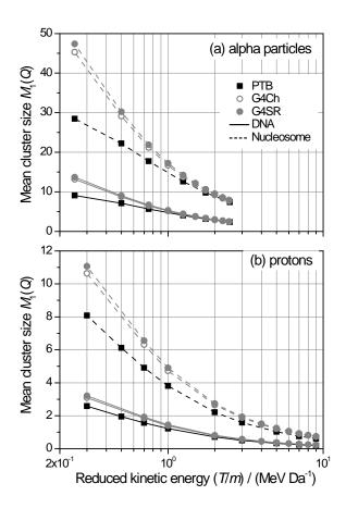
Figure 9. Mean cluster size,  $M_1(Q)$ , as a function of reduced kinetic energy for incident and alpha particles (a) and protons (b), obtained in the DNA segment and the nucleosome by means of Geant4-DNA and PTB MC code.
