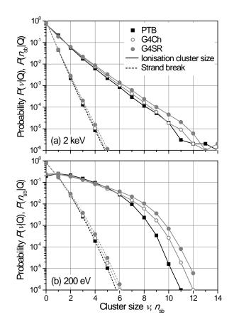
Figure 5. Probability distribution P(v|Q) of ionisation cluster size, v, in the DNA segment and probability distribution,  $P(n_{sb}|Q)$ , for DNA strand break cluster size,  $n_{sb}$ , for 2 keV (a) and 200 eV (b) electrons, calculated by means of the PTB and Geant4-DNA codes using the Screened Rutherford (G4SR) and the Champion model (G4Ch) for elastic scattering.
