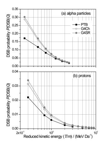
Figure 12. Probability of producing a DSB for alpha particles (a) and protons (b), calculated by means of the PTB and Geant4 MC codes using the Champion model for elastic scattering.
