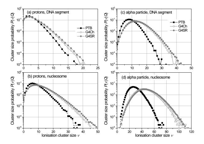
Figure 7. Probability distribution of ionisation cluster size for protons in the DNA segment (a) and the nucleosome (b) obtained for incident protons of 300 keV and incident alpha particles of 1 MeV (c) and (d), calculated by means of the PTB and Geant4 MC codes using the Screened Rutherford (G4SR) and the Champion model (G4Ch) for elastic scattering of the secondary electrons produced. Statistical error bars are not shown; for probabilities of
