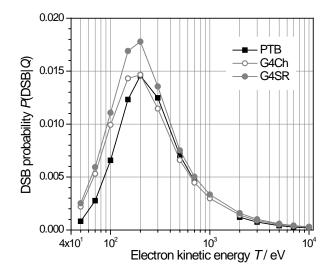
Figure 6. Probability of producing a DSB in the DNA segment as a function of kinetic energy, *T*, calculated by means of the PTB and Geant4 MC codes using the Screened Rutherford (G4SR) and the Champion model (G4Ch) for elastic scattering.
