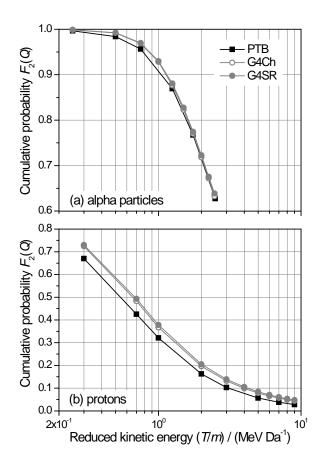
Figure 10. Cumulative probability to produce at least two ionisations within the DNA segment,  $F_2(Q)$ , as a function of reduced kinetic energy for alpha particles (a) and protons (b) calculated by means of PTB and Geant4-DNA MC codes.
