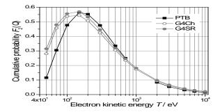
Figure 4.Cumulative probability,  $F_2(Q)$ , for electrons to produce at least two ionisations within the DNA segment, as a function of kinetic energy *T*, for PTB and Geant4 Monte Carlo simulations using the Screened Rutherford (G4SR) and the Champion model (G4Ch) for elastic scattering.
